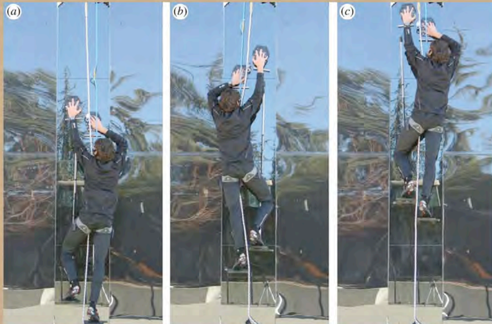
Three frames from a video (electronic supplementary material, move S1) showing a 154 lb climber ascending a 12 ft vertical glass surface using a synthetic adhesion system with degressive load-sharing and gecko-inspired adhesives. The time between (a) and (c) is about 90 seconds and includes six steps.
